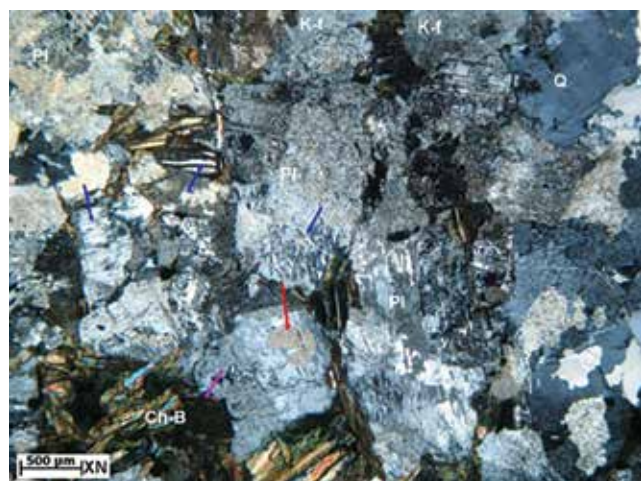
Figure 2. Mineralogy of gradiorite from XRD Red arrows: calcite, blue arrows: zeolite, pink arrow: chlorite.
