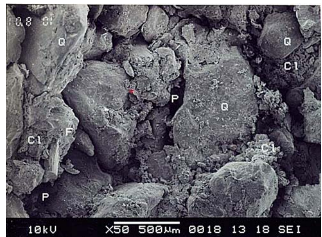
Fig.8. Pore spaces infilled by clay minerals, but still with good connectivity (ST-3X well)
