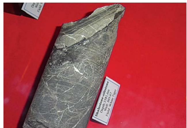
Fig.9. Early Oligocene sandstone highly fractured - Bach Ho field fractures filled by secondary minerals
