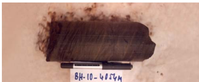
Fig.2. Fine to medium-grained sandstone oil-saturated moderately sorted with cross-bedding point bar facies - Early Oligocene - BH-10 well - 4,054m
